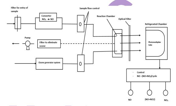
Figure 2: Chemiluminescence Analyzer
