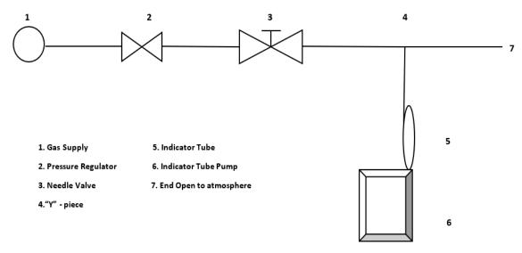
Figure 3: Apparatus for gas detector tube
