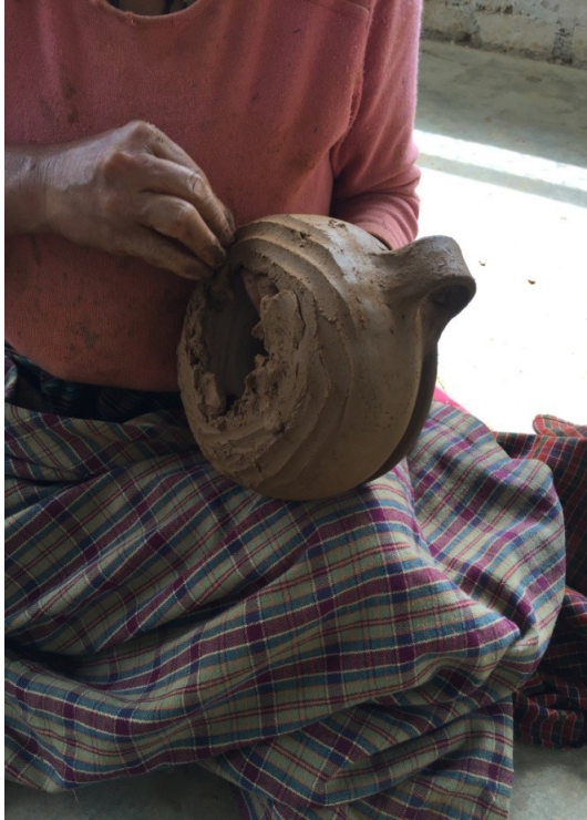
Picture 5: Making the base using additional dough
