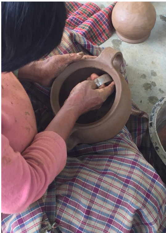
Picture 7: Finishing the inner surface using zharma (ring ribbon tool)
