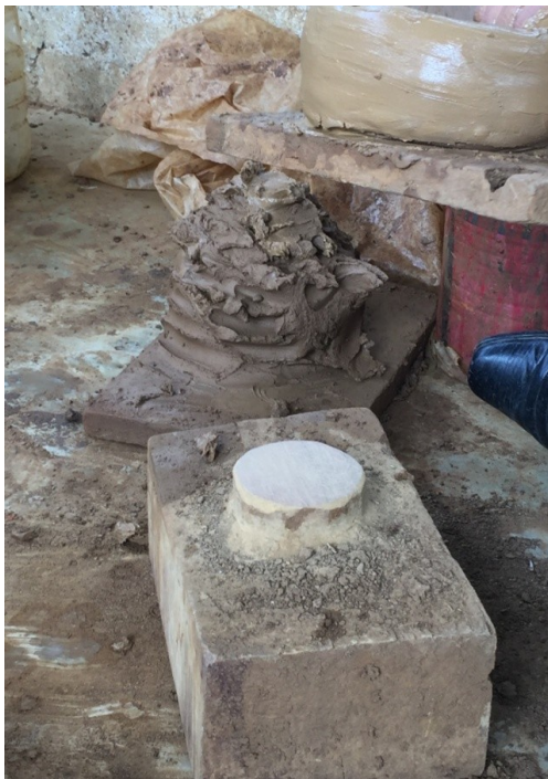
Picture 3: Taypa (wood block with protruding cylinder)
