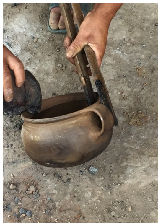
Picture 10: Applying lachaon the product which is taken out of the fire using kempa
