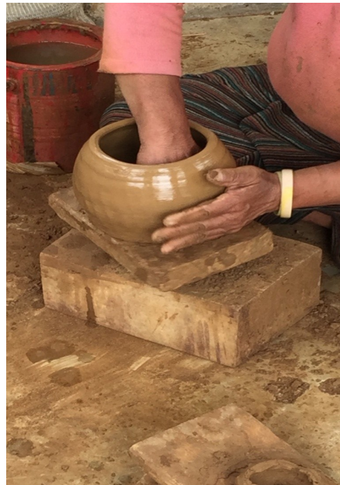
Picture 4: Dipping water on the outer surface to enhance and smoothing the surface
